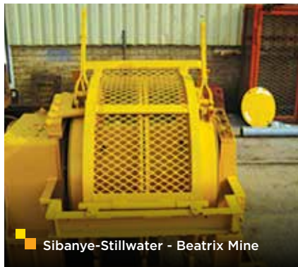
Scraper winch cover before
