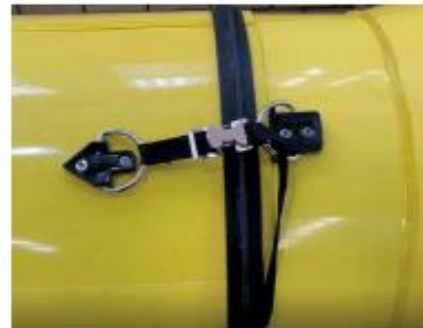
Picture 5. HardLine Coupling Mechanism (over a re-enforcement ring)
