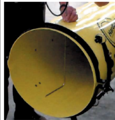
Picture 11. Example of measuring with the pitot tube
