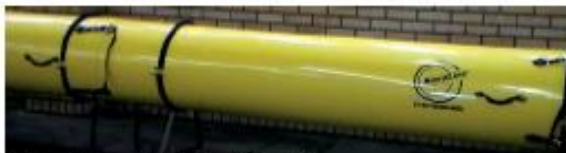
Picture 3. Assembled HardLine duct
