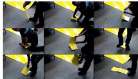
Picture 7. Demonstration of Duct Strength
