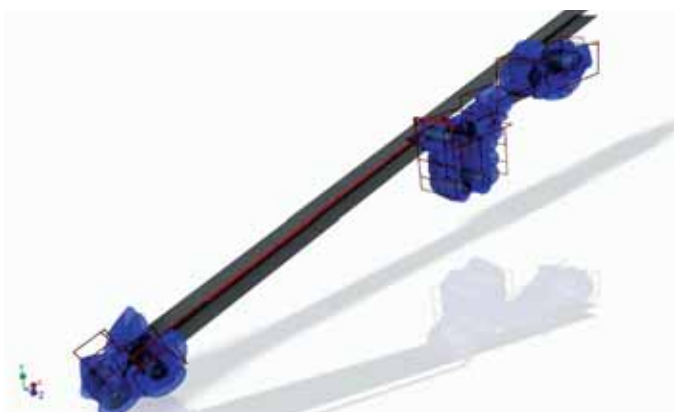
Figure 10: Model of spray patterns for a typical conveyor belt installation.
