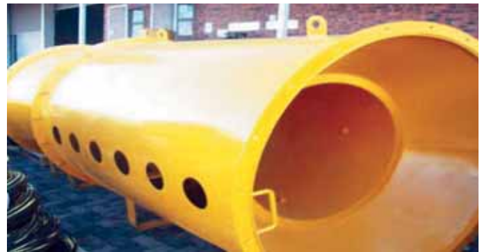
Figure 22: Ventilation column cassette
