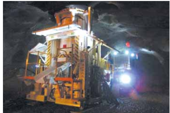
Figure 12: Reef boring machine
