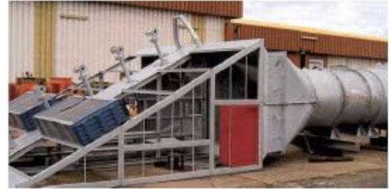
Figure 5. Bank of cooling coils
