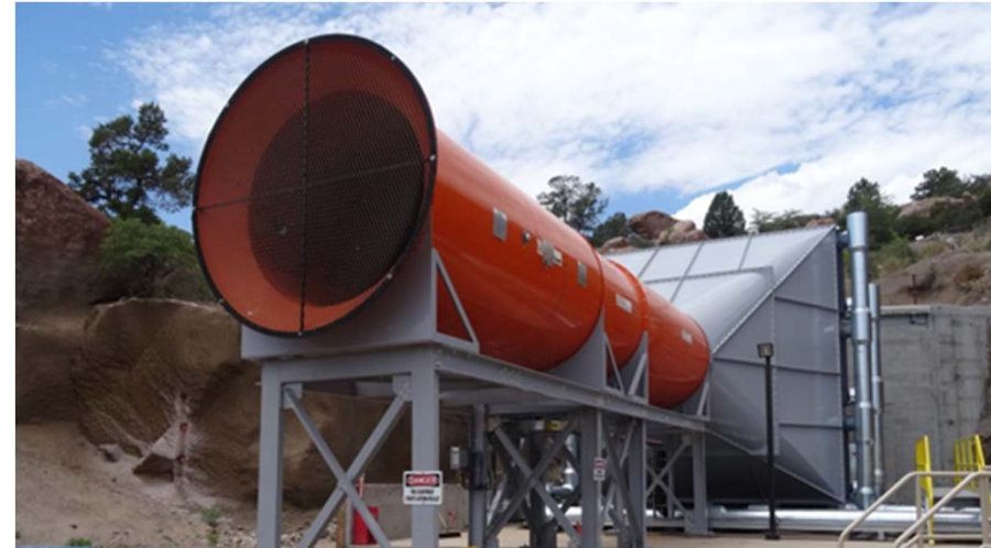
Figure - Example of temporary bulk air cooler
