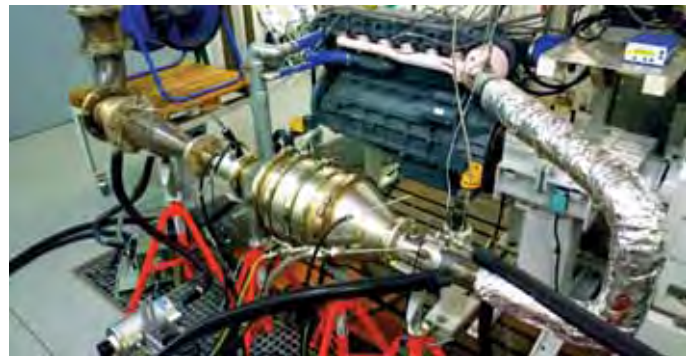
Figure 2. SMF-AR diesel particulate filter fitted to the engine in a test cell at the Sasol Fuels Application Centre
