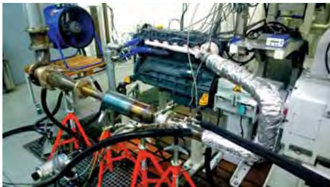
Figure 1. SMF-CRT diesel particulate filter fitted to the engine in a test cell at the Sasol Fuels Application Centre
