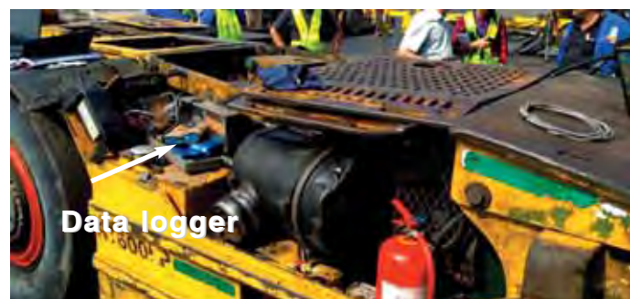
Figure 3. Data logger mounting position on LHD at Bathopele mine in Rustenburg
