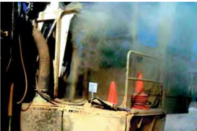
Figure 5. Dust escaping the sealing ring where the drill stem enters the drill deck
