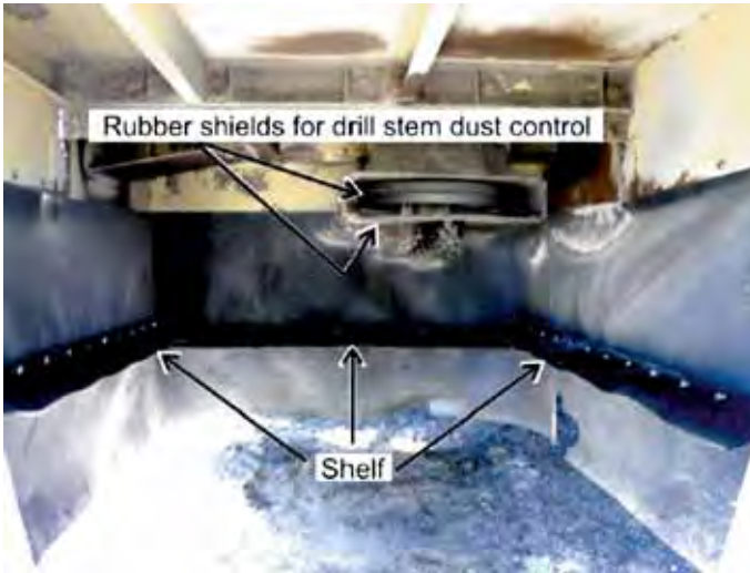
Figure 2. Air-blocking shelf installed along the inside perimeter of the shroud (Cecala et al., 2012)
